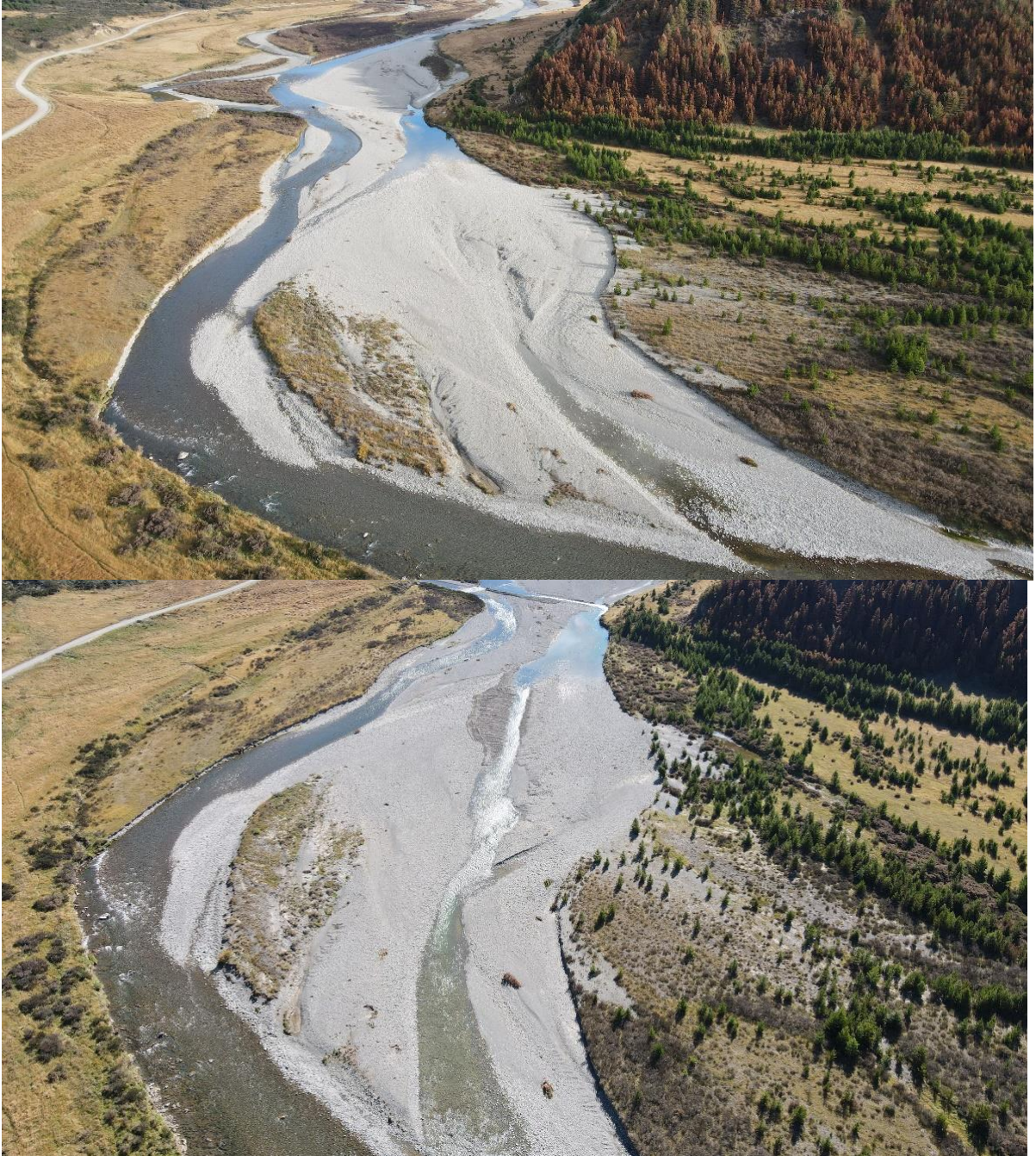
Figure 4. Before (upper) and after (lower) images of Cow Island. River flow was diverted upstream to allow river flow down true left side and along newly cleared and widened channel (true left side of Cow Island).
