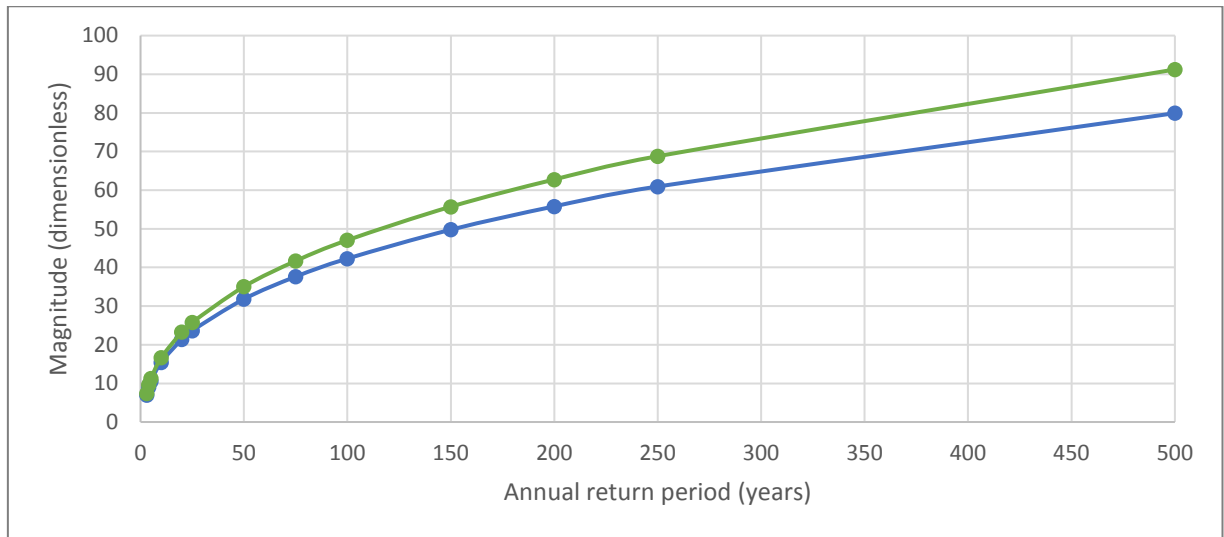
Figure 8.11 Design estimates for magnitudes below 70 m 3 /s. The green line shows results for the time series post-abstraction, the blue line is the pre-abstraction series.
