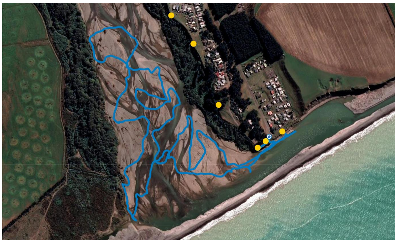
Figure 1. Survey observation points (yellow dots) and GPS-tracking showing a typical route (blue line).
