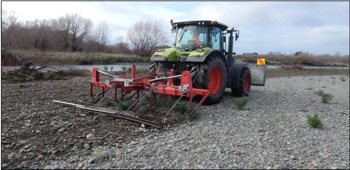
Figure 3: Tractor pulling purpose-built undercutting bar for mechanical weed control on the Ashley Rakahuri River. Photo: Nick Ledgard.
