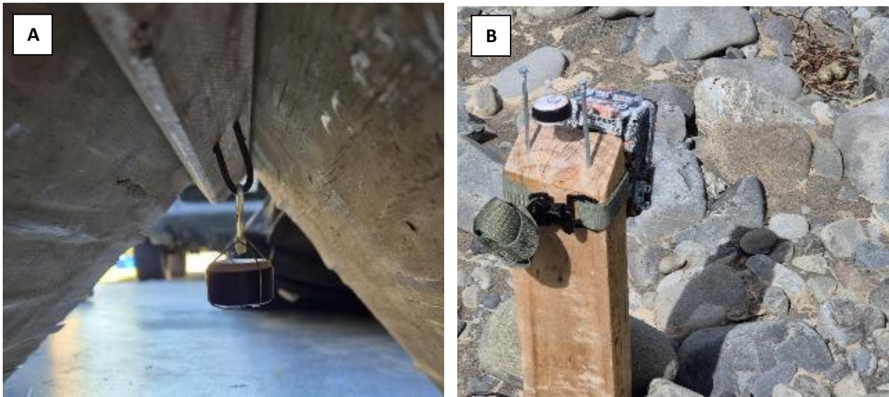
Figure 2: How temperature loggers were attached to A) chick shelters to measure temperature under the shelter and B) camera stands to measure ambient temperature during the 2025/26 tarapirohe season.
