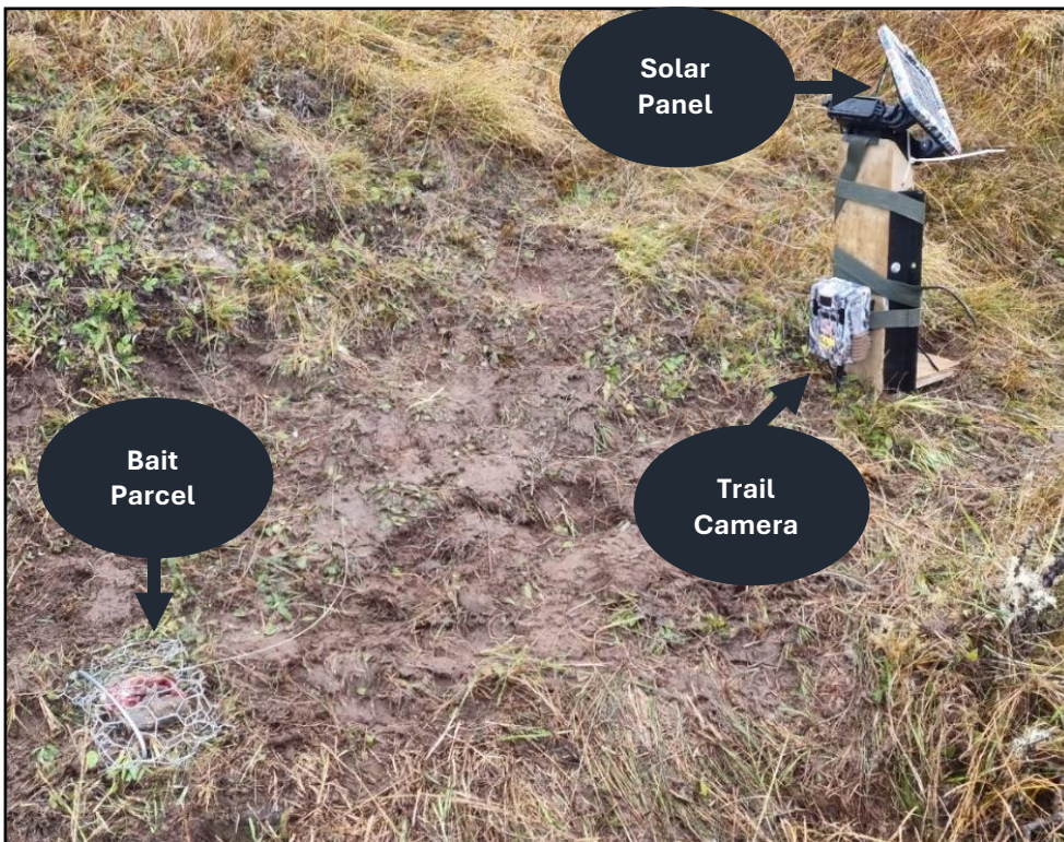
Figure 2: Layout of camera trap station, including solar panel, trail camera and bait parcel. © WMIL.
